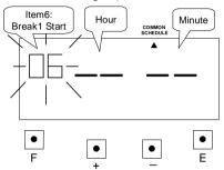
Press the [+] or [-] button to set at "06" and press [E] button. At the same time, the flashing changes from "Item6" to "Hour".
