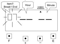
Press the [+] or [-] button to set at "07" and press [E] button. At the same time, the flashing changes from "Item7" to "Hour".
