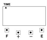
(3) If you want to set another function, press the [F] button to continue setting. If you finished setting the functions, replace the cover and lock it.
