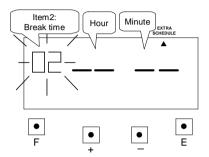
Press the [+] or [-] button to set at "02" and press [E] button. At the same time, the flashing changes from "Item2" to "Hour".
