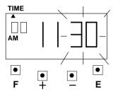
At the same time, the "Second" starts to run from "00" and the LCD screen only display "\( \Delta \)" under the "TIME" mark.
