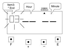
Press the [+] or [-] button to set at "03" and press [E] button. At the same time, the flashing changes from "Item3" to "Hour".
