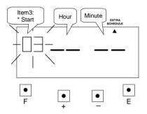
Press the [+] or [-] button to set at "03" and press [E] button. At the same time, the flashing changes from "Item3" to "Hour".
