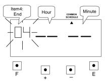
Press the [+] or [-] button to set at "04" and press [E] button. At the same time, the flashing changes from "Item4" to "Hour".
