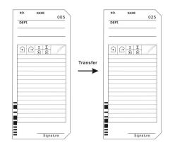
3) Insert the time card No. 25 or press the "+" or "-" button to 025 (card number) then press "E" button. The card number is changed, this mode is complete.
