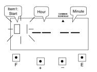
Such as example, press the [E] button because the item is not to be changed. At the same time, the flashing changes from "Item1" to "Hour".
