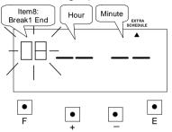
Press the [+] or [-] button to set at "08" and press [E] button. At the same time, the flashing changes from "Item7" to "Hour".
