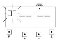
g. Setting the Item7 (Break1 End) **Example:** end time for break1 is set at 10:15.
