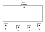
(4) If you want to set another function, press the [F] button to continue setting. If you finished setting the functions, replace the cover and lock it.
