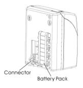
(3) Insert the battery pack into the time recorder as show in the figure.
