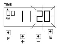
(2) **Setting the "Minute"**Press the [+] or [-] button to set at "30" and press [E] button
